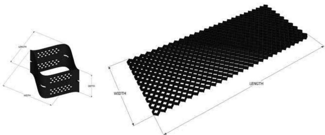
Shahriyar.B.A utilizes interconnected strips of polymer, meticulously welded together at intervals to form a robust and flexible mattress. Filled with granular material, the resulting cellular confinement system efficiently transfers compressive and tensile stresses from heavy loads, providing higher load support capacity than any other geosynthetic product available.
