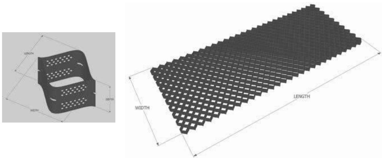
StrataWeb® utilizes interconnected strips of polymer, meticulously welded together at intervals to form a robust and flexible mattress. Filled with granular material, the resulting cellular confinement system efficiently transfers compressive and tensile stresses from heavy loads, providing higher load support capacity than any other geosynthetic product available.
